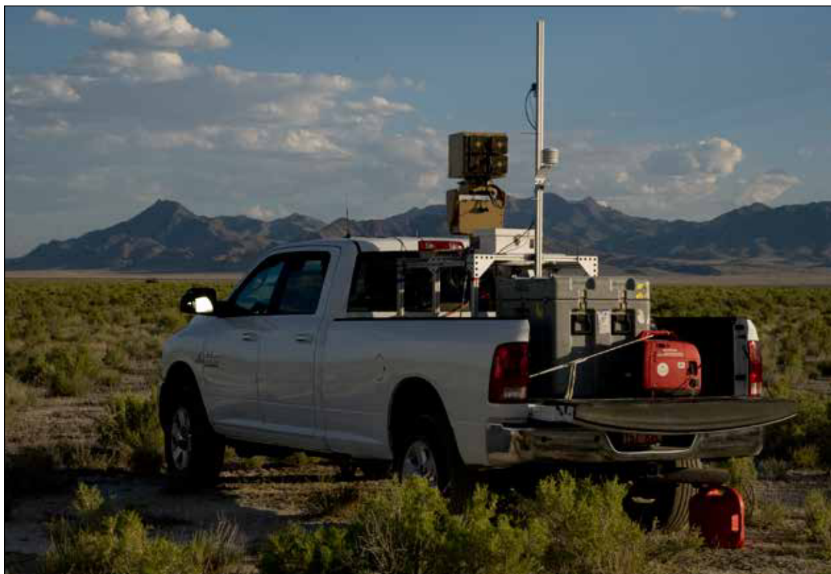
Physical Sciences Inc. of Andover, Mass., demonstrated its Analytic Infrared Imaging Spectroradiometer (ARIS). The mobile unit uses passive infrared to search for biological or chemical agents.
