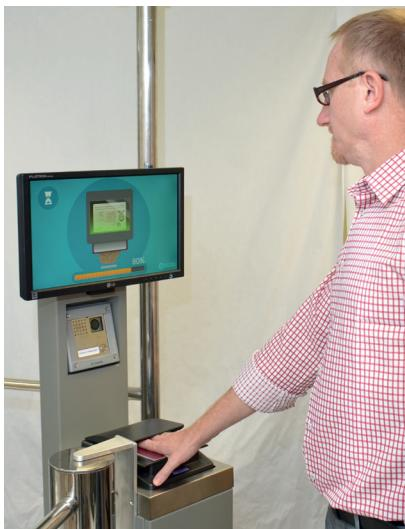
The ABC system compares the fingerprint and face photograph coded in a biometric passport with the same data directly registered from the passenger. Additionally, the possibility that this document can be forged can be analyzed by this system in three spectral ranges. Applying this solution in practice will increase border traffic control and will contribute to the improved safety of EU borders. The ABC system was developed in cooperation with two companies: Optel and MLabs.
