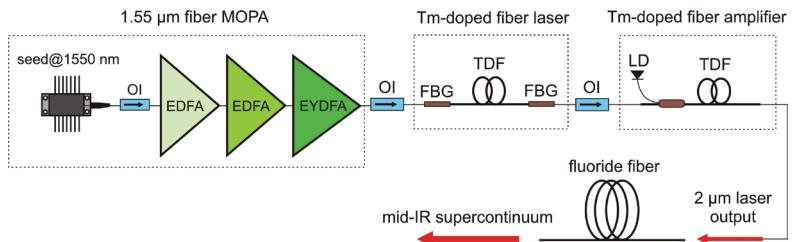
**Figure 1.** Scheme of Tm fiber Master Oscillator and Amplifier
