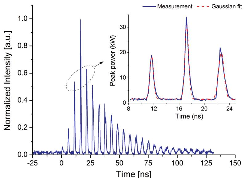
**Figure 2.** Train of optical pulses for pumping the ZBLAN fiber in process of SC generations
