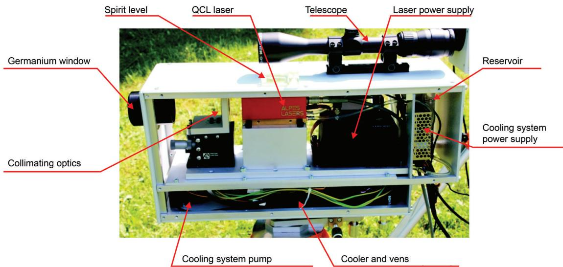
Photo of the FSO transmitter module
