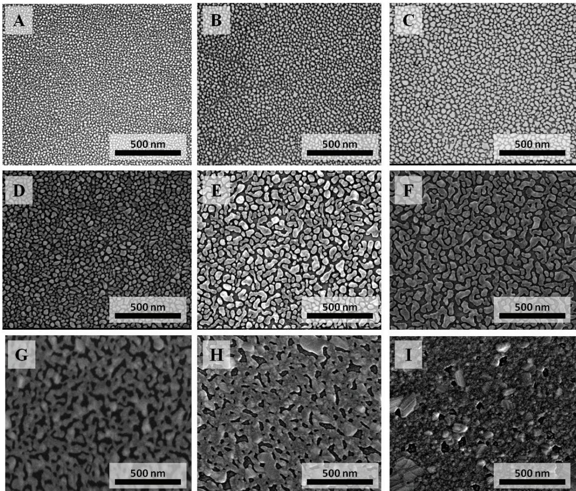
Scanning electron microscope images of silver films with different mass thicknesses
