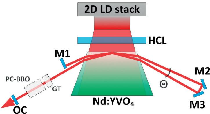
**Figure 1.** Scheme for the Nd:YVO<sub>4</sub> laser with double bounce resonator: HCL - cylindrical lens, OC - output coupler, PC-BBO - Pockels cell, GT - polarizer
