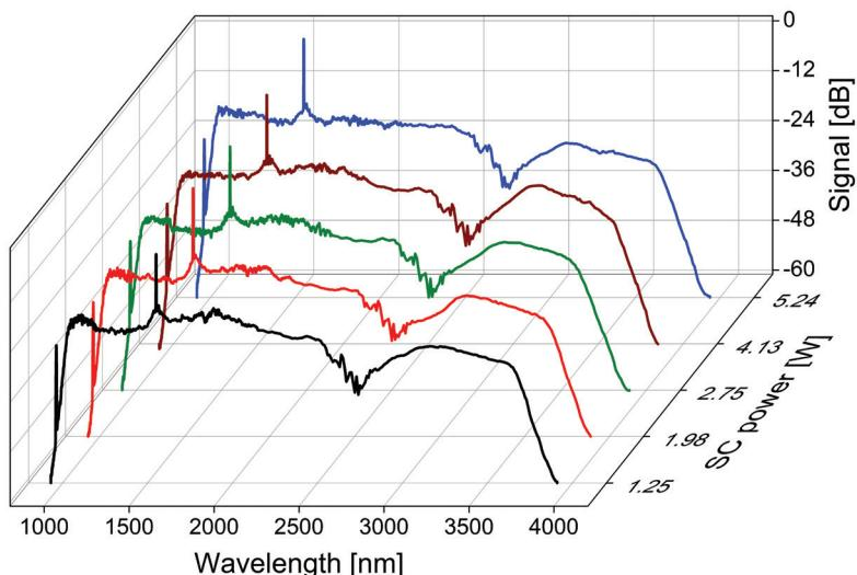
**Figure 2.** Spectrum of SC generation in ZBLAN fiber for different powers up to 5.24 W
