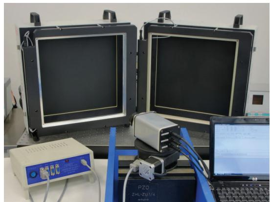
Automatic test stand for the measurement of basic characteristics and calibration of infrared cameras. a) With linear motion module, b) with rotary table
