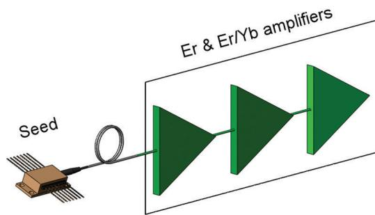
**Figure 1.** Scheme and photograph of ‘eye-safe’, pulsed fiber laser system emitting at 1,55  $\mu$ m
