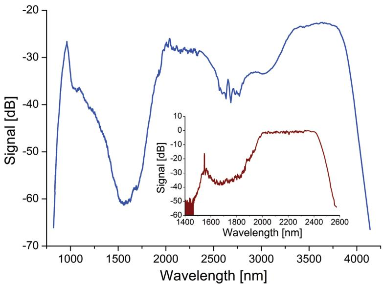
**Figure 1.** Spectrum of SC generation in ZBLAN fiber at output power of 2.24 W
