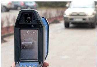
An integrated system of a laser speedometer and image acquisition unit was developed. The formal requirement for these devices is a capability for simultaneously acquiring a speed measurement and a corresponding image (or video) showing the vehicle measured.
