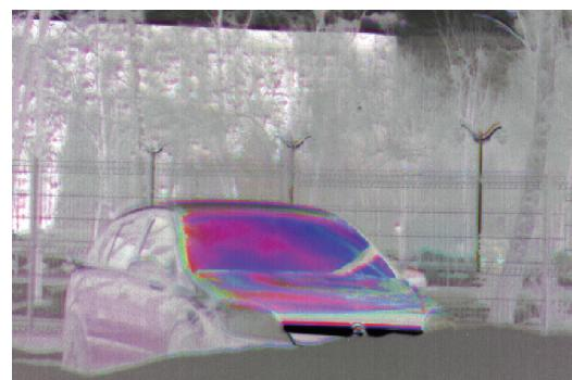
b) Visualization of polarization state measurement results in the LWIR range
