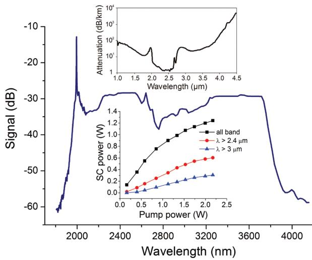
**Figure 3.** Spectrum of SC generation in ZBLAN fiber
