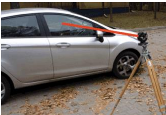
A configuration of the experimental setup, with the reflecting mirror placed on the other side of the car to redirect the laser beam.
