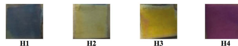
Fig. 4.7.2. Different color anodic titanium oxide layers fabricated by electrochemical oxidation of titanium.
