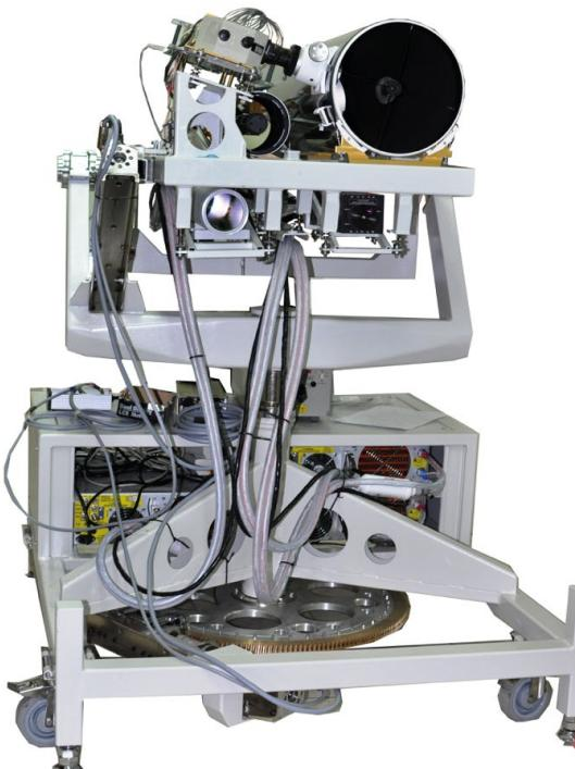
**Fig. 3.** Photo of the Bio-LIDAR
