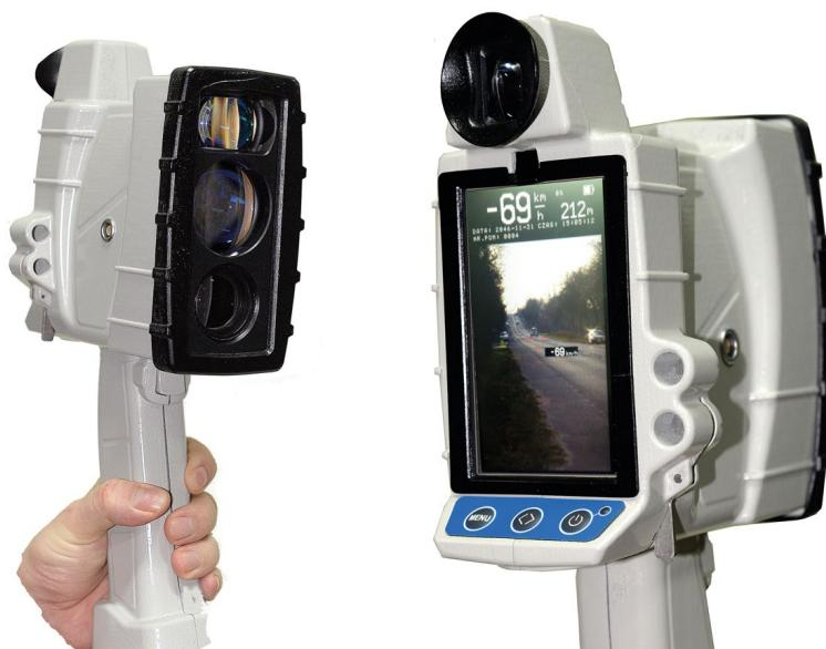
**Fig. 1.** Photos of hand held photo-speedometer
