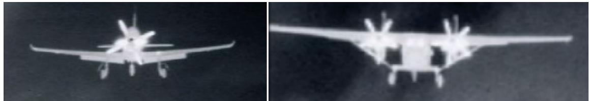
**Fig. 2.** Sample aircraft images recorded from 2 kilometer distance: PZL-130 Orlik, MWIR camera (left), PZL M28B Bryza, LWIR camera (right). Visibility 1 kilometer (light fog)
