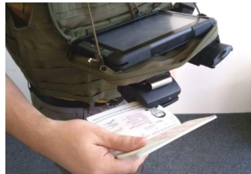
Safety data verification is done through communication with the server certificates. The system is equipped with an experimental ultrasonic fingerprint reader. Work is underway on the possibility of using Augmented Reality technology for data acquisition and visualization of information (HMD module).
