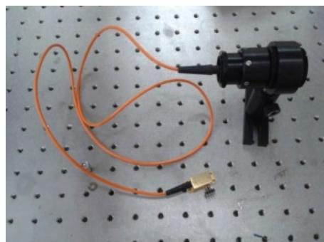
**Fig. 2.** Photo of the laser head with the pumping laser diode
