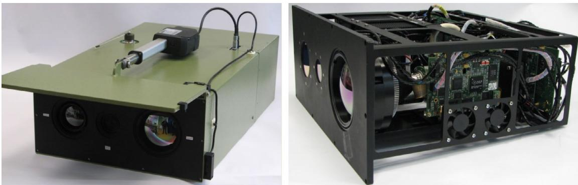
**Fig. 1.** Photo of the set from the camera lens side (from left to right: MWIR, VIS, LWIR) and an inside view with casing removed
